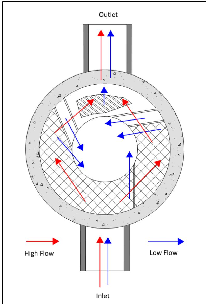
**Figure 1. Hydroworks HydroStorm Operation – Plan View**
