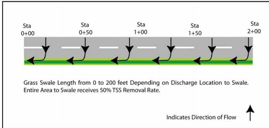
Figure 6.5-2C below shows that from 50 to 150 feet, the inflow area passes through a minimum of 50 feet. Therefore, 100 feet of roadway is treated by a minimum of 50 feet of grass swale. However, from 0 to 50 feet, the inflow area passes through a length of swale less than the 50 foot minimum. Therefore, only the area from 50 feet to 150 feet receives the 50% TSS removal rate.
