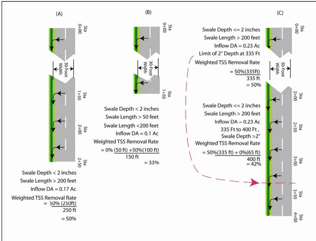
**Note:** Although the last 65 feet of the roadway in Figure 6.5-4(c) does not receive water quality credit, it may qualify as a vegetated conveyance for the purposes of demonstrating the use of nonstructural stormwater management strategies.
